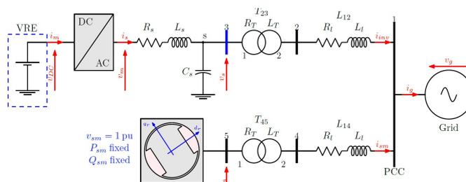
Figure 1: A synchronous machine and a power electronics converter jointly participate to energy production on power grid
