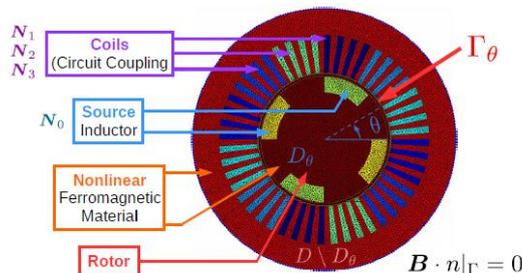
Figure 1: Finite Element Model for an electrical machine
