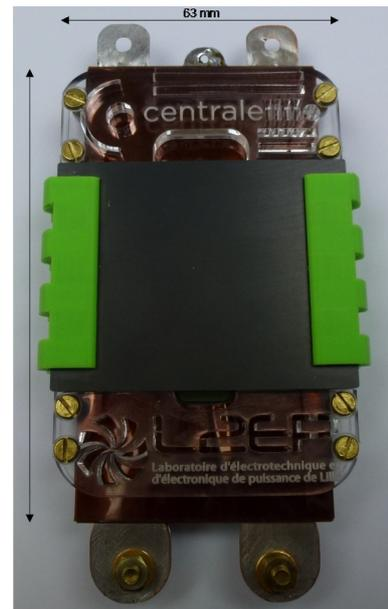
**Fig.1: 2.5 kW 2-winding planar transformer**
